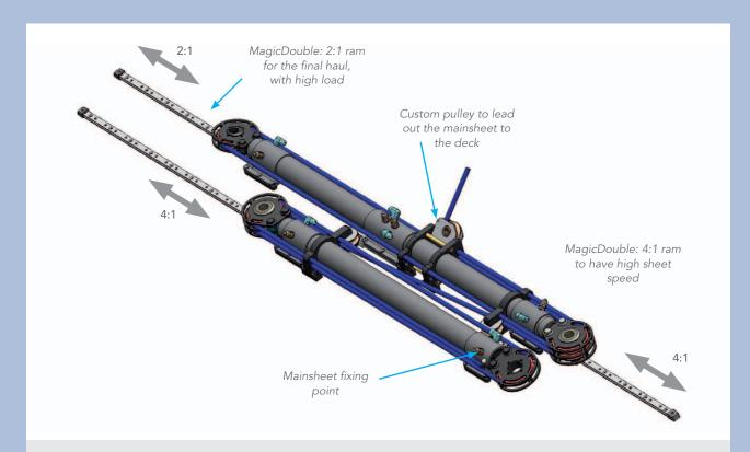
The mainsheet Magic Trim + Magic Double system developed for a Swan '60. Trim sequence: both cylinders closed, Magic Trim start to exit, than starts the 4:1 side of Magic Double tacking the mainsheet speed. When the 4:1 side of Magic Double is fully extended and the load of sheet increases, the 2:1 Magic Double ram completes the hauling of the sheet. Vice versa for easing sequence.
