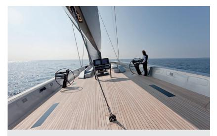
Wally 130' deck: Smart MagicTrim and MagicDouble are used for mainsheet and jib sheet. Thanks to these automatic systems, the deck is flush and free from winches and their sheets.
