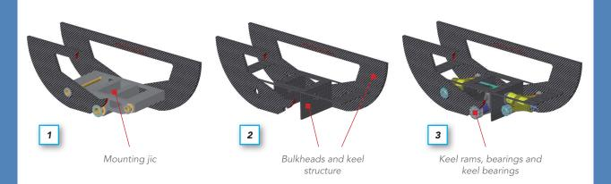
Here above you can see how the shipyard made the structural part of the canting keel system.
