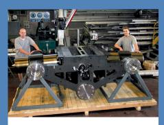
Cariboni's keel system with frame for a 105' sloop. This kind of system is fully tested in the firm before shipping.
